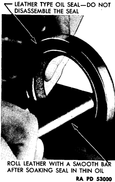
Figure 155—Conditioning Oil Seal
