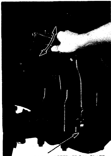
LINK DISCONNECTED FROM PLATE PUMPING
