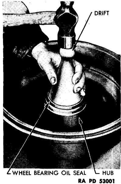
Figure 156—Installing Wheel Bearing Oil Seal with Drift 41-D-1535-50
